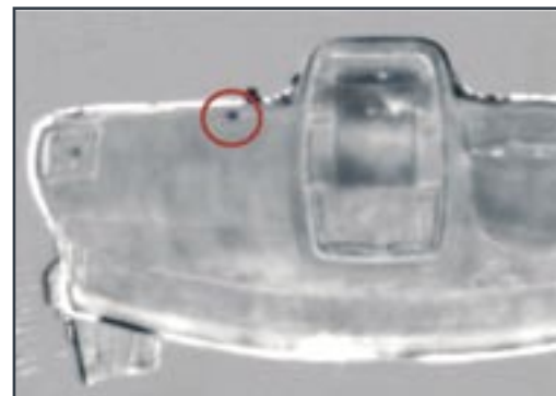
Result image showing cavities in the foam
