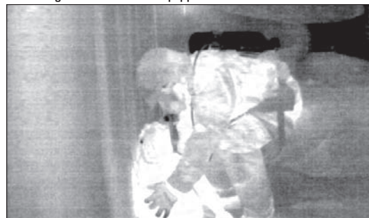
IR image through thick smoke.
